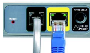
Figure 3-4: Connect to the Ethernet Port
